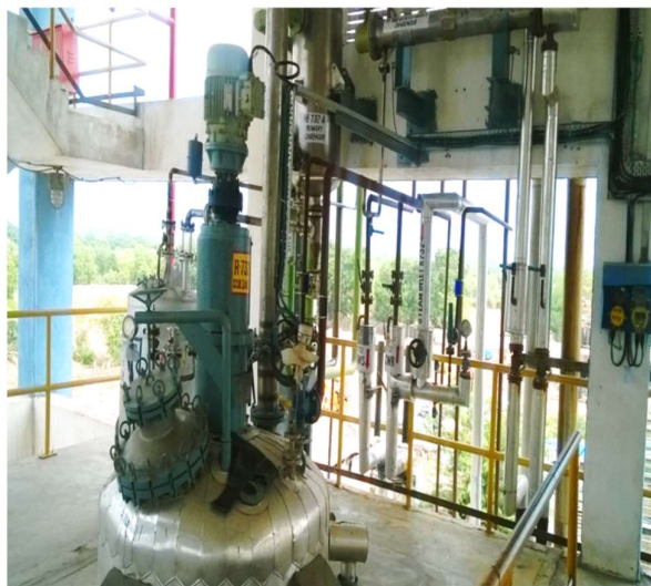
Primary And Secondary Condensers for VOC control
